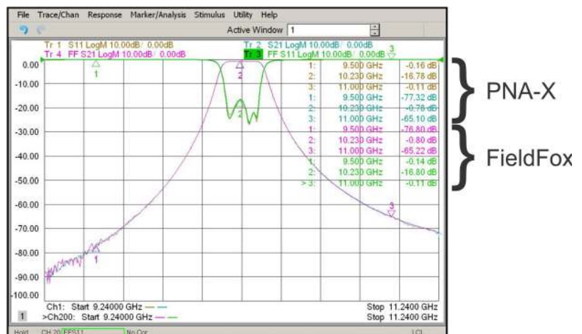
Figure 1. S11 and S21 for a 10 GHz filter measured using a PNA-X benchtop vector network analyzer (VNA) and a FieldFox VNA
